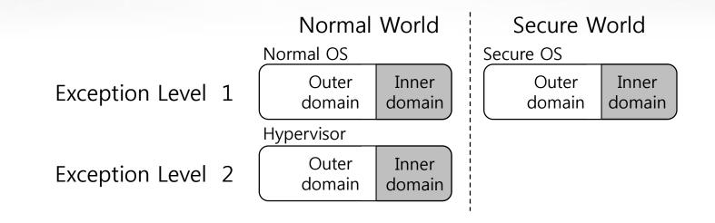
To achieve the goal of Hilps, two core mechanisms for intralevel isolation and domain switching must be applicable regardless of exception level
