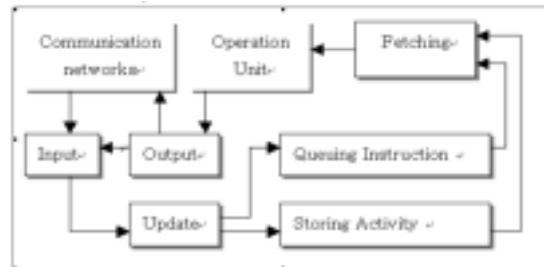
Figure 1.4 A simple model of a processing element for a static data flow machine
